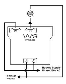
Note: Incase of Mains Supply failure, Load L1 will work on Backup Supply.
